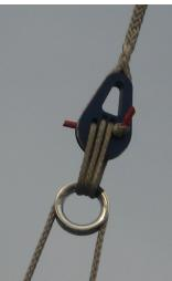
Static lashing block lashed to a Line Terminator.
